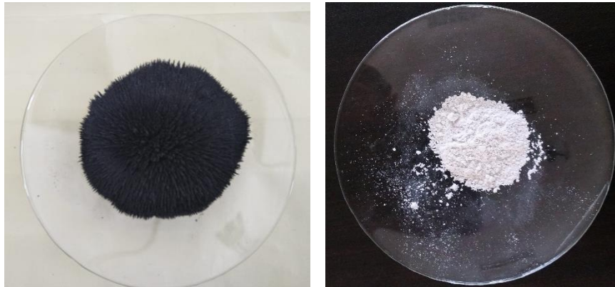
Gambar 1. (a) Hasil preparasi pasir besi Pantai Kendal, (b) Adsorben nanomaterial hibrida PB@SiO_2@TA
