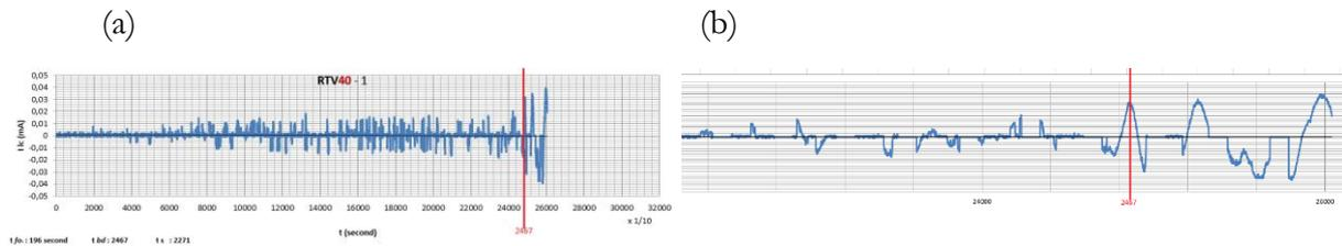
**Figure 7.** a) Leakage current test results for the RTV40 resin epoxy composite sample 1. b) Results of 10x magnification range before breakdown
