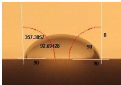
*Figure 3. Calculation of the sample contact angle*
