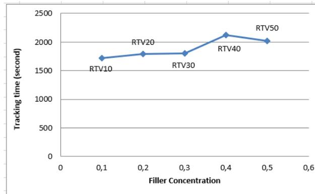
**Figure 8.** Graph of the relationship between tracking time and the concentration of composite fillers
