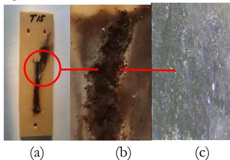
**Figure 9.** Photographs (a) without magnification (b) macro 10 $\times$  and (c) macro 30 $\times$  from the surface of the RTV30 epoxy resin composite sample
