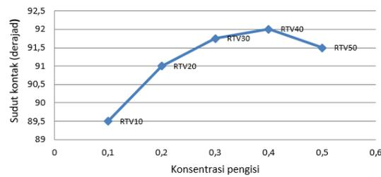
Figure 6. Graph of relationship between contact angle and filler concentration of epoxy resin composites
