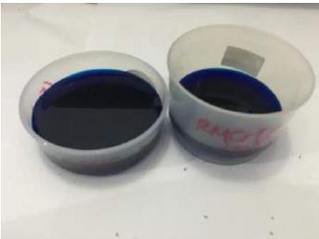
Gambar 4. Perendaman dalam *methylene blue* 4 jam
