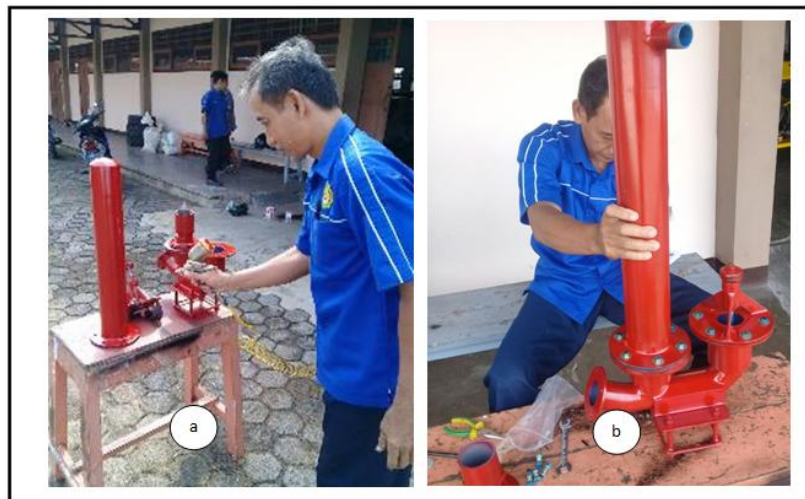
Gambar 3: (a) Coating Anti Karat, (b) Set-up Pompa Hidram
